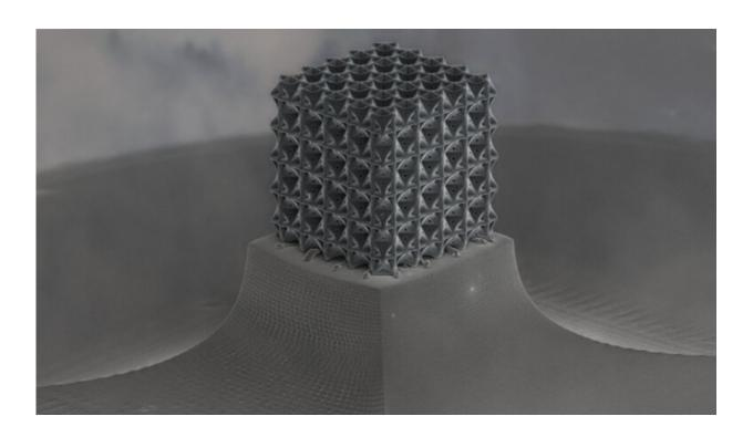
With wall thicknesses of about 160 nanometers, a closed-cell, plate-based nanolattice structure designed by researchers at UCI and other institutions is the first experimental verification that such arrangements reach the theorized limits of strength and stiffness in porous materials. Credit: Cameron Crook and Jens Bauer / UCI
