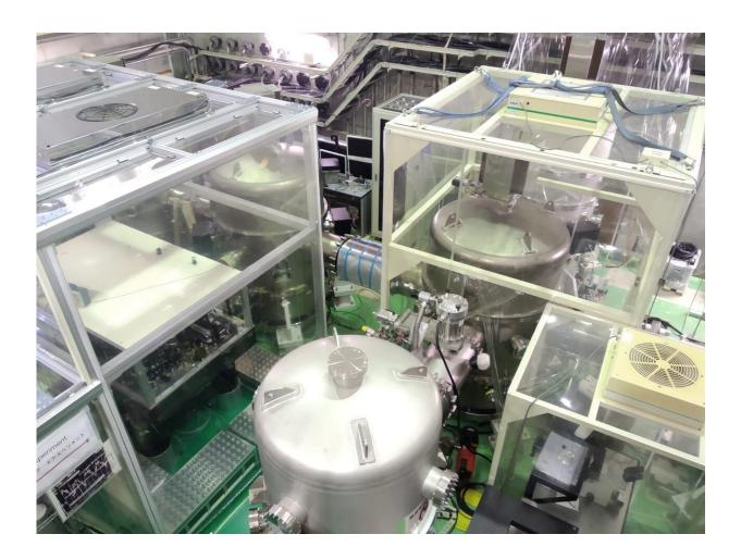
Vacuum chambers in the infrastructure of the former TAMA300 detector used in this experiment. Credit: NAOJ
