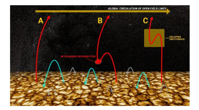
Illustration of global magnetic field circulation enabled by interchange reconnection. In this scenario an open magnetic field line is (A) dragged against
