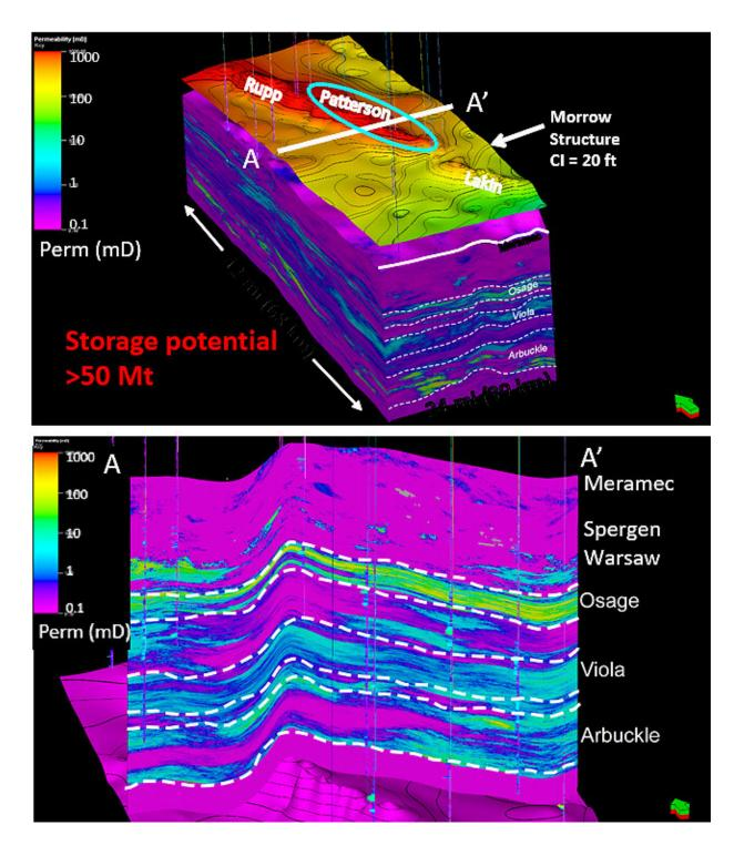
The 3-D model (top) shows storage potential of rock layers from the top of the Meramec formation—more than 4,000 feet deep in Kearny County—to the top of the basement. The map above is the top of the Morrow formation overlying the Meramec. The cross section (bottom) shows formations underlying line A-A'
