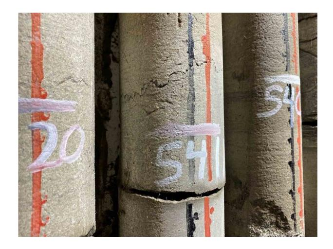
Cores pulled up from more than 5,400 feet beneath the surface at the IMSCS-HUB well site in Kearny County. Credit: University of Kansas
