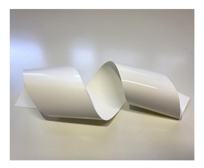
The team say that the mechanical robustness and operability of the flexible composite sheet at a wide range of temperatures makes it a promising electrolyte for Li-metal batteries. Credit: Tokyo Metropolitan University
