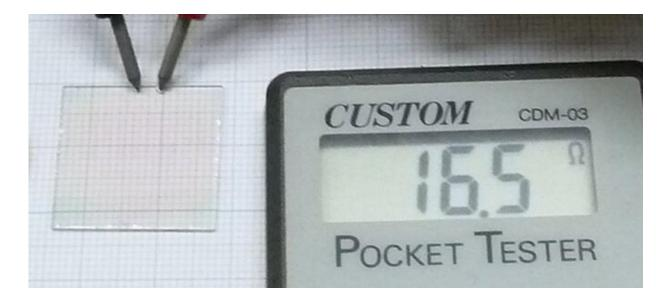
The final tin dioxide thin film grown on glass to make efficient photovoltaics. Credit: © 2020 Nakao et al.
