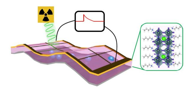
X-ray detectors made with 2-dimensional perovskite thin films convert X-ray photons to electrical signals without requiring an outside power source, and are a hundred times more sensitive than conventional detectors. Credit: Los Alamos National Laboratory
