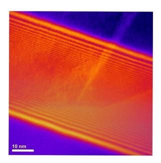
Seeing the invisible: An electron hologram of a grain boundary in a lightly doped solid electrolyte sample from which electric potential at the grain boundary can be recovered. Credit: Argonne National Laboratory
