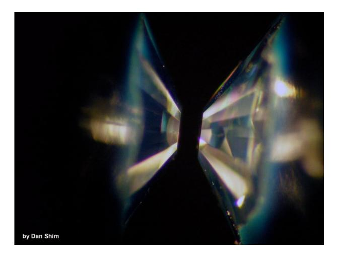
In a diamond-anvil cell, two gem quality single crystal diamonds are shaped into anvils (flat top in the photo) and then faced with each other. Samples are loaded between the culets (flat surfaces), then the sample is compressed between the anvils. Credit: Dan Shim/ASU
