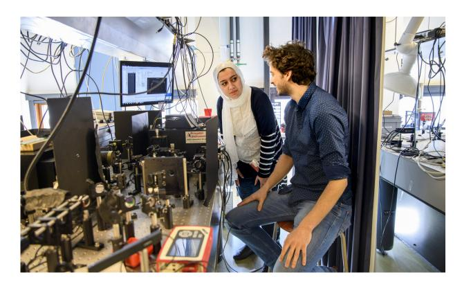
Shared first authors Elham Fadaly (left) and Alain Dijkstra (right) operating an optical setup to measure the light that is emitted. The emission from the hexagonal-SiGe alloy showed to be very efficient and suitable to start producing an all-silicon laser. Credit: Sicco van Grieken, SURF
