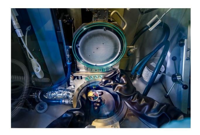
A look inside the Metal Organic Vapor Phase Epitaxy (MOVPE). This machine was used to grow nanowires with hexagonal silicon-germanium shells. The emission from this hexagonal-SiGe alloy showed to be very efficient and suitable to start producing an all-silicon laser. Credit: Nando Harmsen, TU/e
