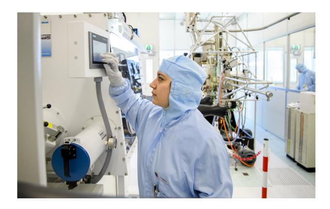
Shared first author Elham Fadaly, is operating the Metal Organic Vapor Phase Epitaxy (MOVPE). This machine grows the nanowires with hexagonal silicongermanium shells. The emission from this hexagonal-SiGe alloy showed to be very efficient and suitable to start producing an all-silicon laser. Credit: Sicco van Grieken, SURF
