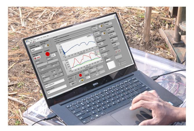
A readout of spectral signatures produced by the team's prototype, which collects the visible and near-infrared wavelengths that bounce back from soils. Credit: Greg Nathan | University Communication
