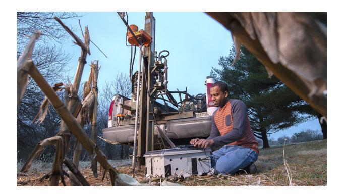
Nuwan Wijewardane, postdoctoral researcher in biological systems engineering, prepares to hydraulically plunge a penetrometer prototype into soil. Credit: Greg Nathan | University Communication
