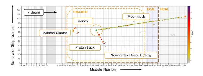
This display shows a CCQE-like event reconstructed in the MINERvA detector. Credit: MINERvA
