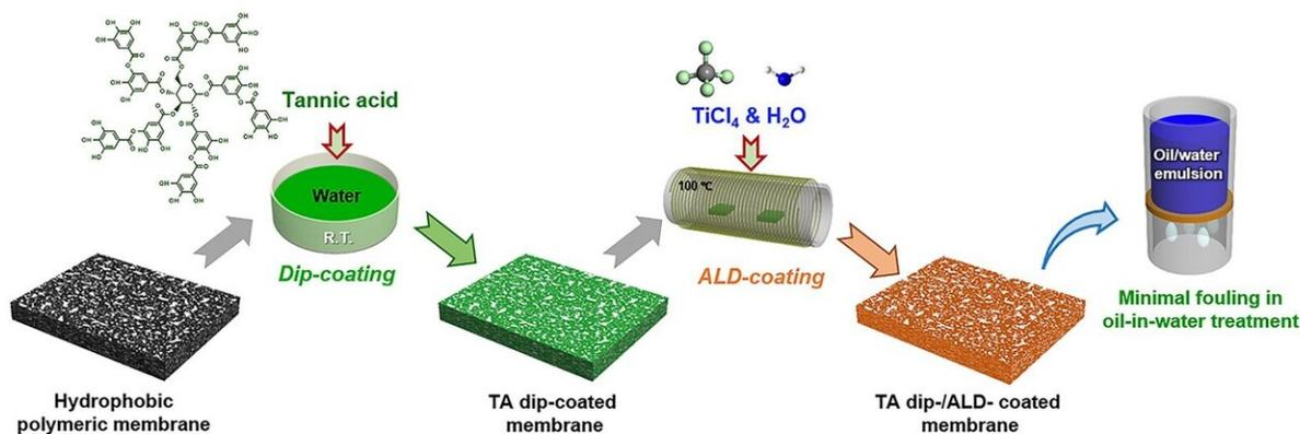
In the experiment, researchers first dip-coated a hydrophobic polymeric membrane in tannic acid (TA), a common polyphenol. Then, the dried TA dip-coated membrane is loaded into the atomic layer deposition (ALD) reactor for coating with titanium dioxide using the precursors titanium tetrachloride and water ( $\text{TiCl}_4$  and  $\text{H}_2\text{O}$ ). The coated membranes display minimal fouling in oil-in-water treatment. Credit: Argonne National Laboratory
