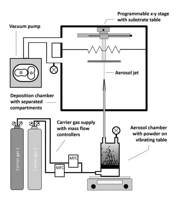
A scheme of the Powder Aerosol Deposition (PAD). Credit: UBT.
