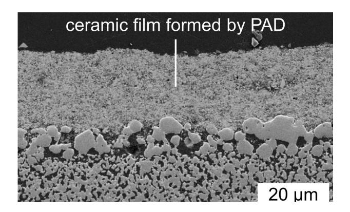
A ceramic film produced by powder aerosol deposition on a porous gaspermeable electrode, such as those required in fuel cells. Credit: Jörg Exner.
