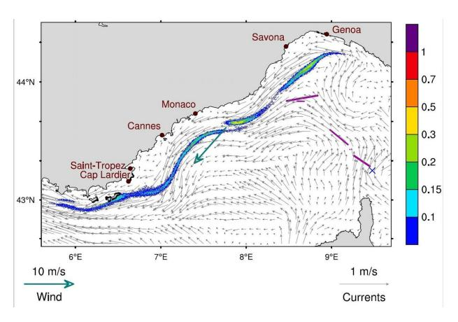
Pink polygons indicate the area where the model was restarted from on 10 Oct. 2018. A blue cross marks the ships' point collision. Credit: ©Svitlana Liubartseva, CMCC Foundation
