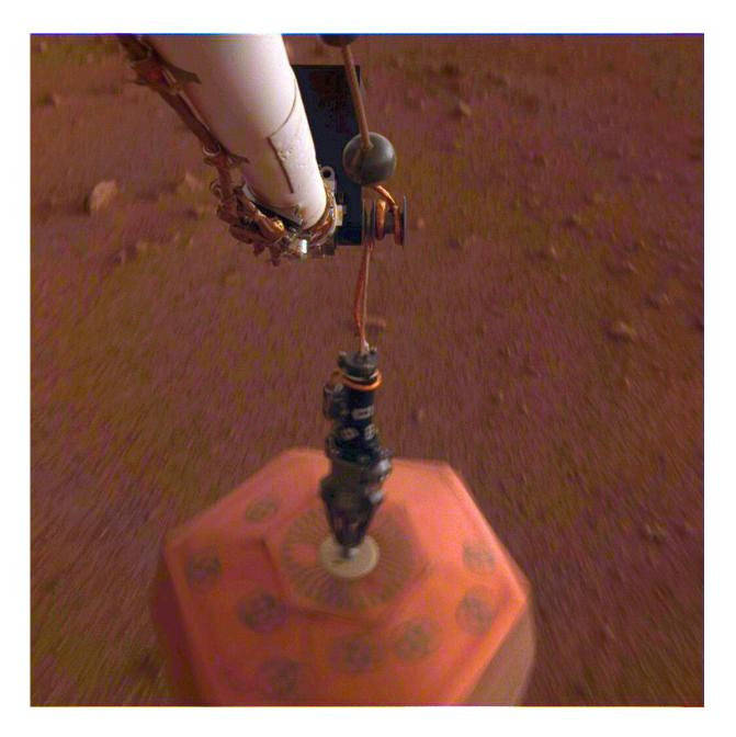
The seismometer on the MarsInsight mission is the most capable to date; however, a deployment arm must position it. Credit: NASA
