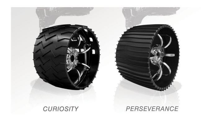
Illustrated here, the aluminum wheels of NASA's Curiosity (left) and Perseverance rovers. Slightly larger in diameter and narrower, 20.7 inches (52.6 centimeters) versus 20 inches (50.8 centimeters), Perseverance's wheels have twice as many treads, and are gently curved instead of chevron-patterned. Credit: NASA/JPL-Caltech
