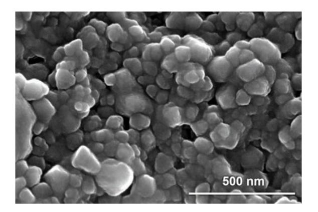
SEM images of lipid-coated MIL-100(Fe) (e) nanoparticles at 150 000× magnification. Credit: Ploetz et al, *Advanced Materials* 2020
