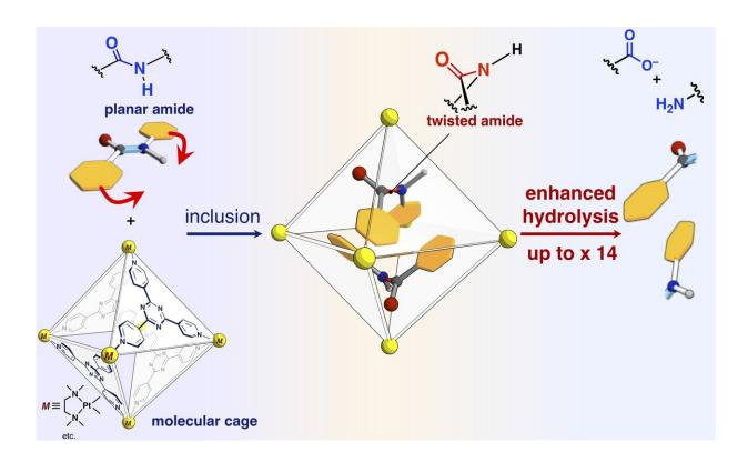
A scheme of reaction rate acceleration of amide hydrolysis by inclusion in the self-assembled molecular cage. Credit: NINS/IMS
