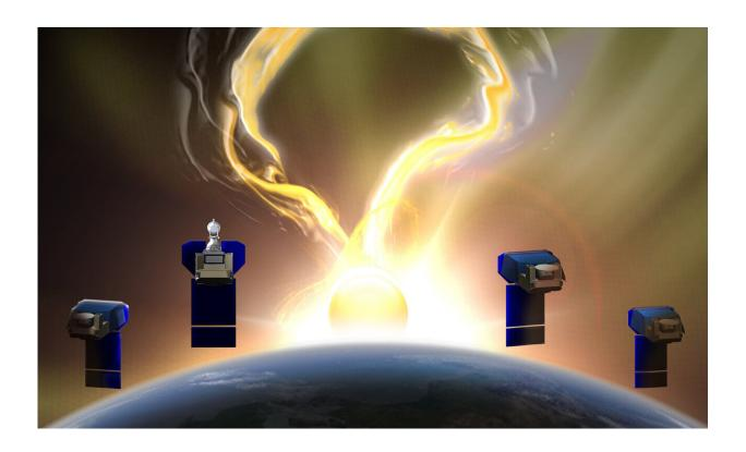
NASA has selected Southwest Research Institute to lead a microsatellite mission to image the Sun's outer corona. PUNCH proposes a constellation of four suitcase-sized satellites that will orbit the Earth, studying how the Sun's corona connects with the interplanetary medium, to better understand how coronal structures infuse the solar wind with mass and energy. Credit: Southwest Research Institute
