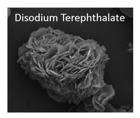
Disodium terephthalate flowers produced from polyethylene terephthalate via microwave processing in two minutes. Purdue University researchers created a technique to turn waste polyethylene terephthalate, one of the most recyclable polymers, into components of batteries. Credit: Vilas Pol/Purdue University
