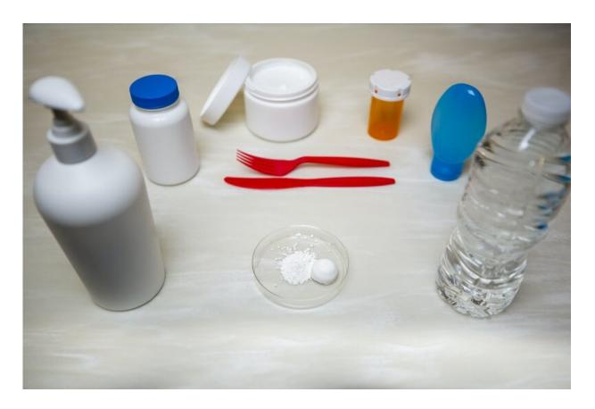
The Circe process uses engineered microbes to produce a powdered form of the polymer PHA (center), which can be processed into a variety of plastic products. Credit: Wyss Institute at Harvard University
