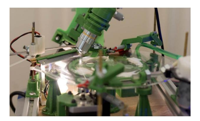
The inside of the pollen trap with the rotating glass plate and the digital microscope. Credit: Nam Cao
