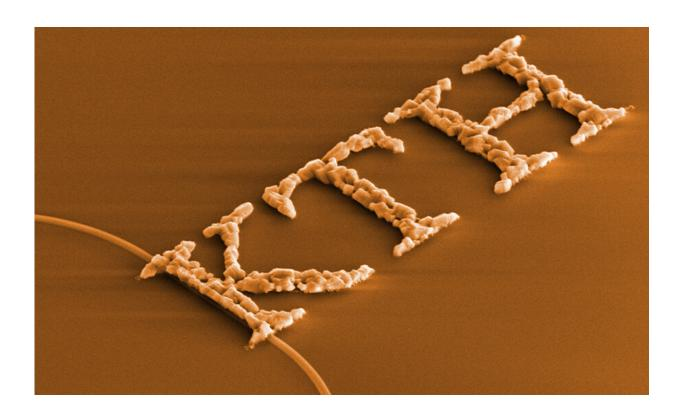
Synthesized copper oxide crystals arranged to spell out the name of the university where the production method originated. Credit: KTH Royal Institute of Technology.
