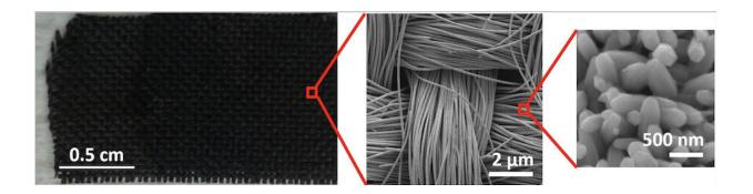
Here's a sample from Sonal Padalkar's lab: a carbon cloth coated with zinc oxide nanomaterials that are just billionths of a meter in size. Padalkar says the shape, size and density of the zinc oxide can be fine-tuned on the cloth. Credit: Sonal Padalkar
