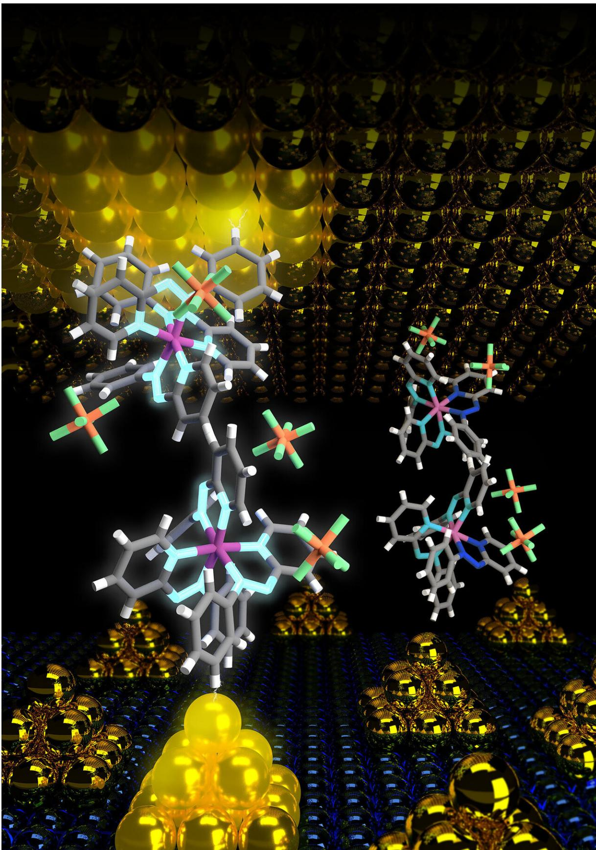
The device structure at a molecular level. The gold nanoparticles on the bottom electrode enhance the field enabling an ultra-low energy operation of the molecular device. Credit: Sreetosh Goswami, Sreebrata Goswami and Thirumalai Venky Venkatesan
