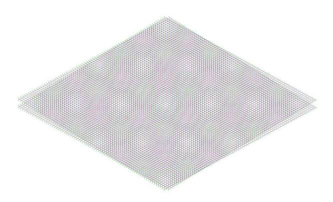
The moiré effect with two lattices placed on top of each other. Theslight twist between the lattices results in a coarser moiré patternwith distant lattice points (light and dark regions). Credit: ETH Zurich / Yuya Shimazaki
