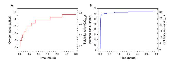
Gas uptake as a function of time. Results shown for oxygen (A) and methane (B) at 60 V (with average field intensity of 12 kV/m), expressed as a multiple of their respective HLCs (right axis) and in g/liter (left axis) at prevailing background pressures of ~90 bar; plateaux occurred within less than 3 hours. Credit: Science Advances, doi: 10.1126/sciadv.aaz0094
