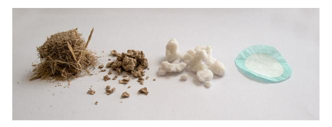
From bagasse to a new nano-particle removing material. Credit: Queensland University of Technology
