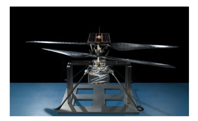
The technology behind the Mars Helicopter's 4-foot-wide (1.2-meter-wide) rotor blades is also used in the construction of a rugged drone that helps farmers survey their land. Credit: NASA/JPL-Caltech
