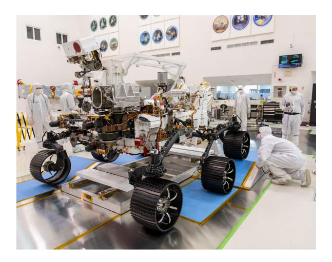
In a clean room at NASA's Jet Propulsion Laboratory in Pasadena, USA, engineers observed the first driving test for NASA's Mars 2020 rover 17 December 2019. Credit: NASA/JPL-Caltech
