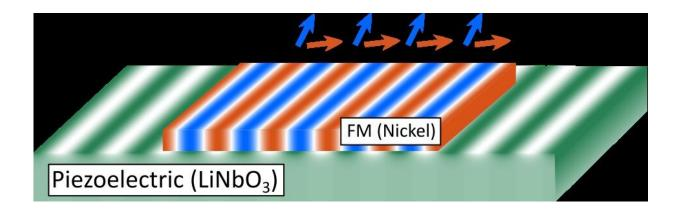
Scheme of the strain caused by the surface acoustic waves (SAWs) in the piezoelectric (in green color scale) and magnetic modulation in the ferromagnetic material (in orange-cyan color scale). Credit: B. Casals et al.
