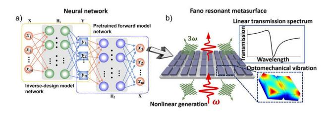
(a) Schematic of a tandem neural-network used for the inverse design of a Fano resonant metasurface for enhancing (b) nonlinear generation and optomechanical vibrations. Credit: SPIE
