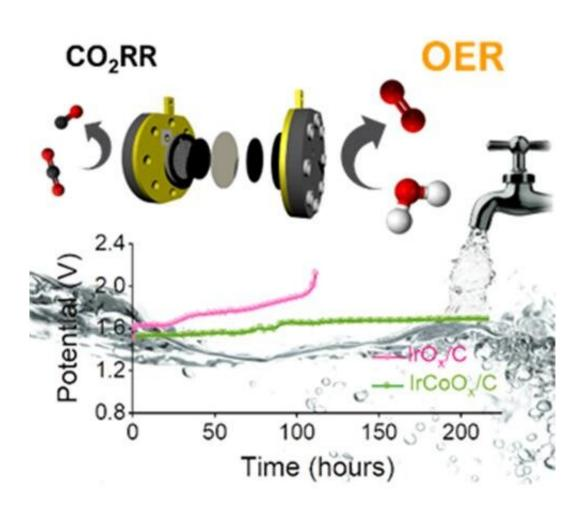
The catalyst developed by KIST's research team uses 20% less iridium, a precious metal, than existing catalysts and shows at least 31% higher performance. A long-term test using tap water was performed to verify the practical feasibility of the catalyst. When tested, the catalyst maintained a high level of performance for hundreds of hours, indicating high durability.When the developed catalyst was applied to the actual carbon dioxide conversion system,
