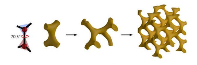
Figure 1: Schematic of the structural units of a single-gyroid network, starting with a pair of vertices which share one of their three struts and are offset by a "twist" angle. The middle image shows how vertex pairs make up one gyroid unit cell, and the right image shows how unit cells assemble into the gyroid network. Credit: Dustin Llandro and David Love and András Kovács
