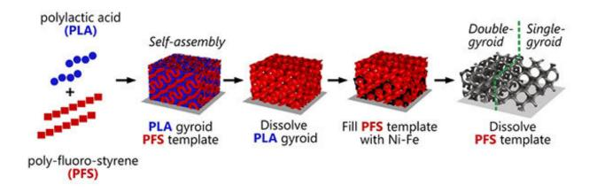
Figure 2: Schematic of the process of producing the Ni-Fe gyroid nanostructures by self-assembly . Credit: []Justin Llandro and David Love and András Kovács
