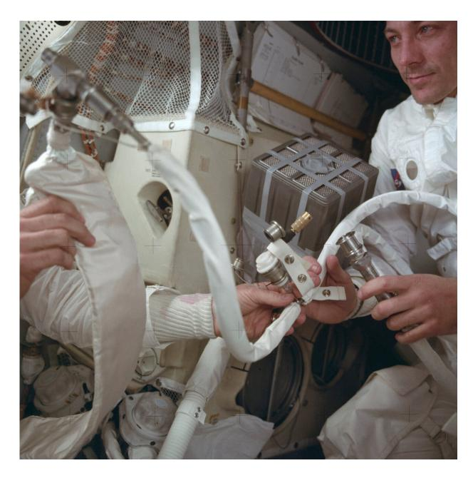
In this April 1970 photo provided by NASA, Apollo 13 command module pilot John Swigert helps to hook up a lithium hydroxide canister in the lunar module, in an effort to get rid of carbon dioxide in the cabin as the spacecraft attempts to return to Earth. The explosion of an oxygen tank in the service module forced the three-man crew to rely on the lunar module as a "lifeboat." (NASA via AP)
