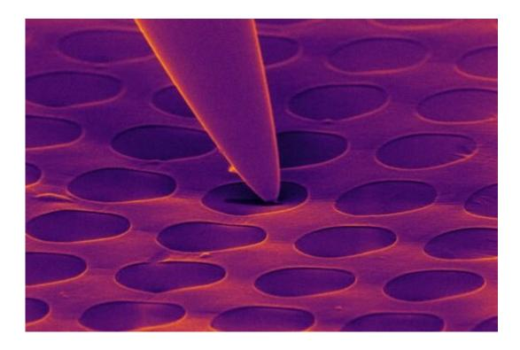
Small metal tip used for cleaning of surfaces on the nanoscale. Credit: CENEM, FAU Erlangen-Nürnberg
