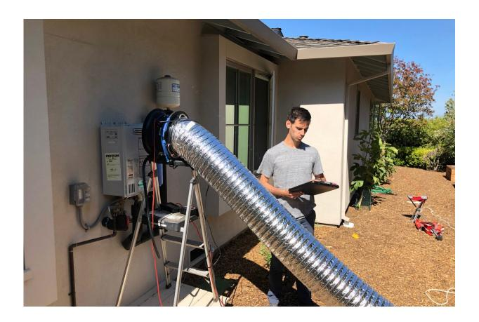
Stanford staff researcher Colin Finnegan records notes as a Duct Blaster captures the methane being emitted from the tankless water heater on the side of a house in the study. Credit: Rob Jackson
