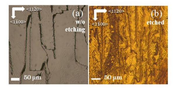
In addition to large grooves, which were present before etching, high density of small grooves were observed on the surfaces after etching. Credit: NITech
