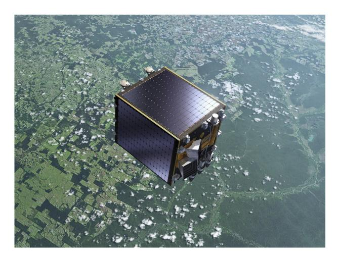
The 'V' in its name stands for Vegetation: Proba-V will fly a reduced-mass version of the Vegetation instrument currently on board the Spot satellites to provide a daily overview of global vegetation growth. The Proba satellites are part of ESA's In-orbit Technology Demonstration Programme: missions dedicated to flying innovative technologies. Credit: ESA-P.Carril
