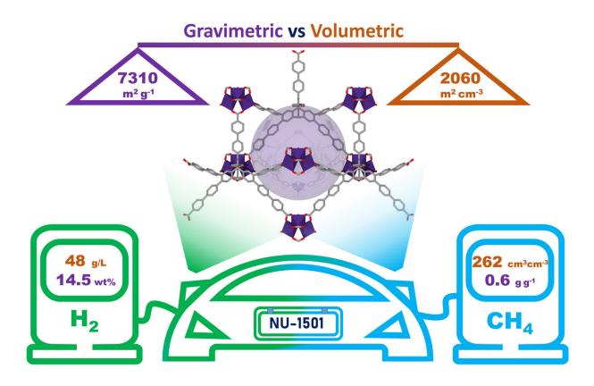
A highly porous material balancing gravimetric and volumetric storage performances. Credit: Timur Islamoglu and Zhijie Chen
