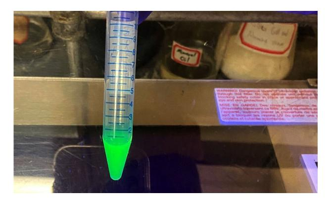
The biosensor created by Shahir S. Rizk of IU South Bend produces a fluorescent light signal that can quantify how much glyphosate is in a sample. Credit: Shahir S. Rizk
