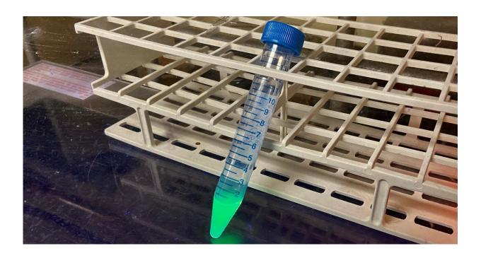
The fluorescent biosensor created by Shahir S. Rizk of IU South Bend can detect glyphosate below the federally mandated levels for drinking water in the U.S. Credit: Shahir S. Rizk
