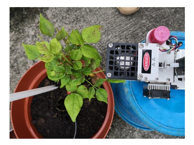
A Li-cor photosynthesis system was used to measure the photosynthetic rate of the plant. Credit: The Chinese University of Hong Kong (CUHK)
