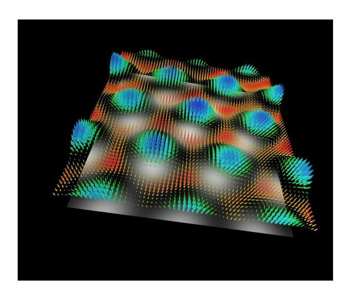
Snapshot of the nanofilm that displays the electric field of light in the plasmonic nanovortices (skyrmions). The hexagonal (6-fold) symmetry in the plane is easily
