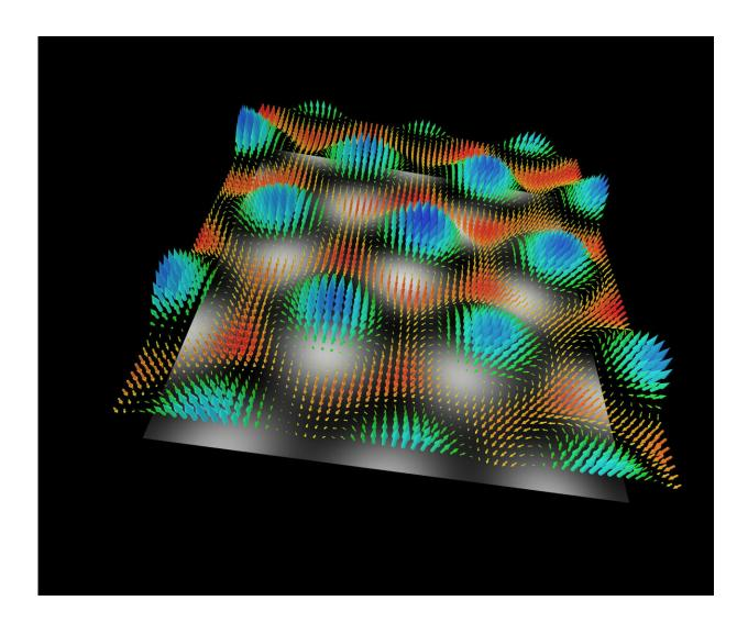
Snapshot of the nanofilm that displays the electric field of light in the plasmonic nanovortices (skyrmions). The hexagonal (6-fold) symmetry in the plane is easily
