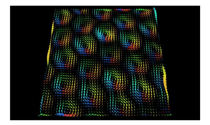
Analogy to nano tornadoes in plasmonic vortices (skyrmions). The display exibits the measured 3-dimensional structure of the magnetic field of the light on the gold nanoplatelets. Credit: University of Stuttgart
