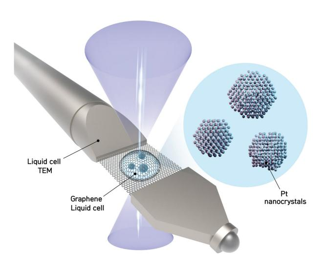
The schematic shows a liquid sample contained between two sheets of graphene -- the thinnest, strongest material known. Nanoparticles in the liquid freely rotate while a transmission electron microscope takes thousands of images of the nanoparticles. The images are then analyzed by the authors' software to determine the location of every atom in each nanoparticle Credit: IBS
