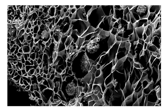
A scanning electron microscope image of the microalgal colonies in the hybrid living biopolymers. Credit: University of Cambridge
