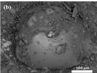
(a) Preliminary tests for the 3-D Printing of lunar regolith simulant NU-LHT-2M on a carbon steel baseplate and (b) SEM image of the same. Credit: Politecnico di Milano
