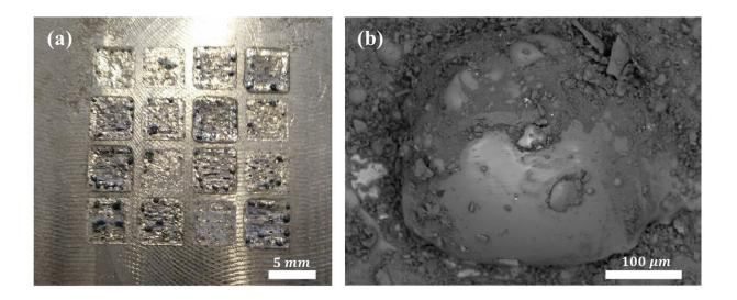
(a) Preliminary tests for the 3-D Printing of lunar regolith simulant NU-LHT-2M on a carbon steel baseplate and (b) SEM image of the same. Credit: Politecnico di Milano
