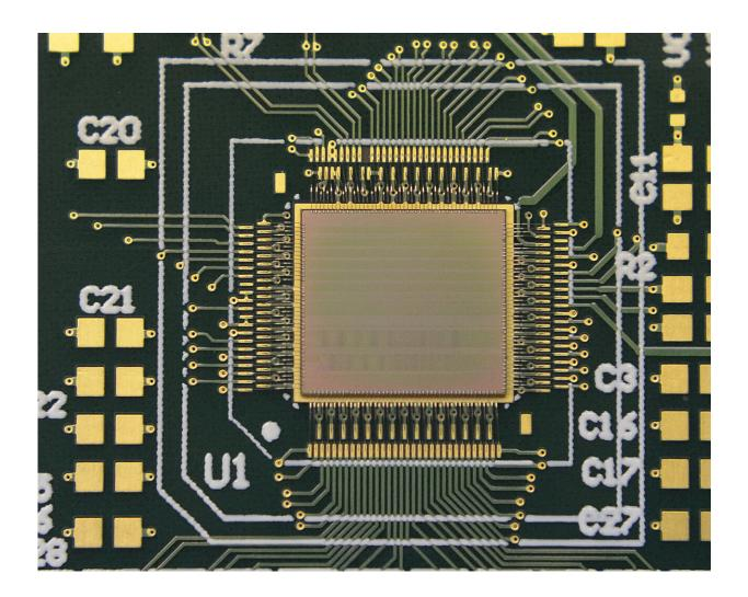
Analog-to-digital convertors built to work at cryogenic temperatures, such as the prototype pictured here, will operate inside of liquid-argon chambers in the Deep Underground Neutrino Experiment. Credit: Alber Dyer, Fermilab
