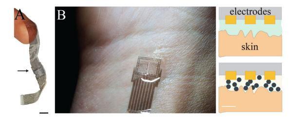
Confirmable electronics and high-quality noninvasive electrophysiological recording by mixed-conducting particulate composites (MCP)A) Micrograph of
