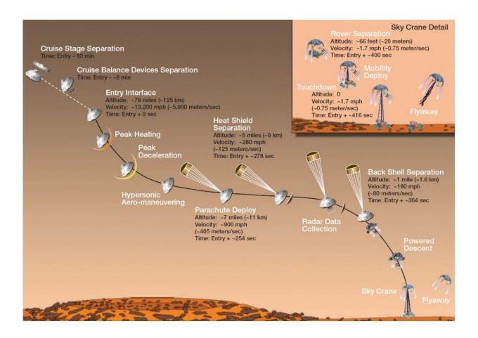
"Seven Minutes of Terror" – the Entry, Descent and Landing (EDL) of the Mars Science Lab (MSL) – Mars Curiosity Rover. China hasn't released all of the details, but they say that their Tianwen mission will also utilize retrorockets and parachute to land on Mars. (Credit: NASA/JPL)
